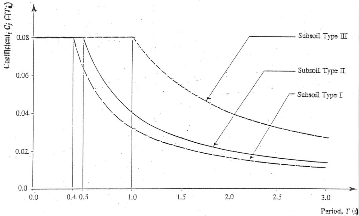
Figure.1: Basic seismic coefficient,  $C$ , and Basic response spectrum,  $C(T_i)$
